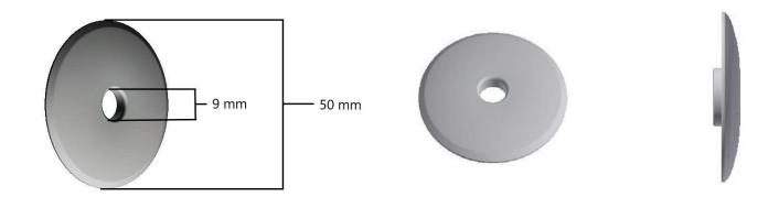
The fastening system FRT consists in a disc made in PA6 grey colour which is fixed on supports through a  $\emptyset$  6 mm, self-drilling, countersunk-head screw or through a  $\emptyset$  6 or  $\emptyset$  8 mm hammer plug. The tightening of the self-drilling screw or of the hammer plug, inserted in the central disc, create the right pressure for fixing the insulation.
